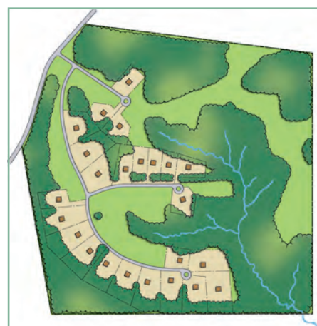
Figure 9 Option 2 Age-targeted Community 25% Density Increase 24 Lots Lot Size: 12,000 to 24,000 sq. ft. 60% Undivided Open Space
