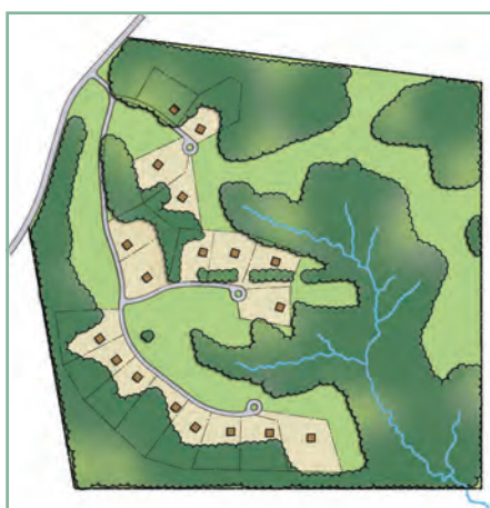
Figure 8 Option 1 Density-neutral 18 Lots Lot Size Range: 20,000 to 40,000 sq. ft. 50% Undivided Open Space
