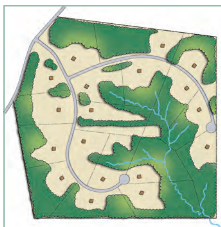
Figure 7 Yield Plan Conventional Development Pattern 18 Lots Min. Lot Size: 80,000 sq. ft. No Undivided Open Space
